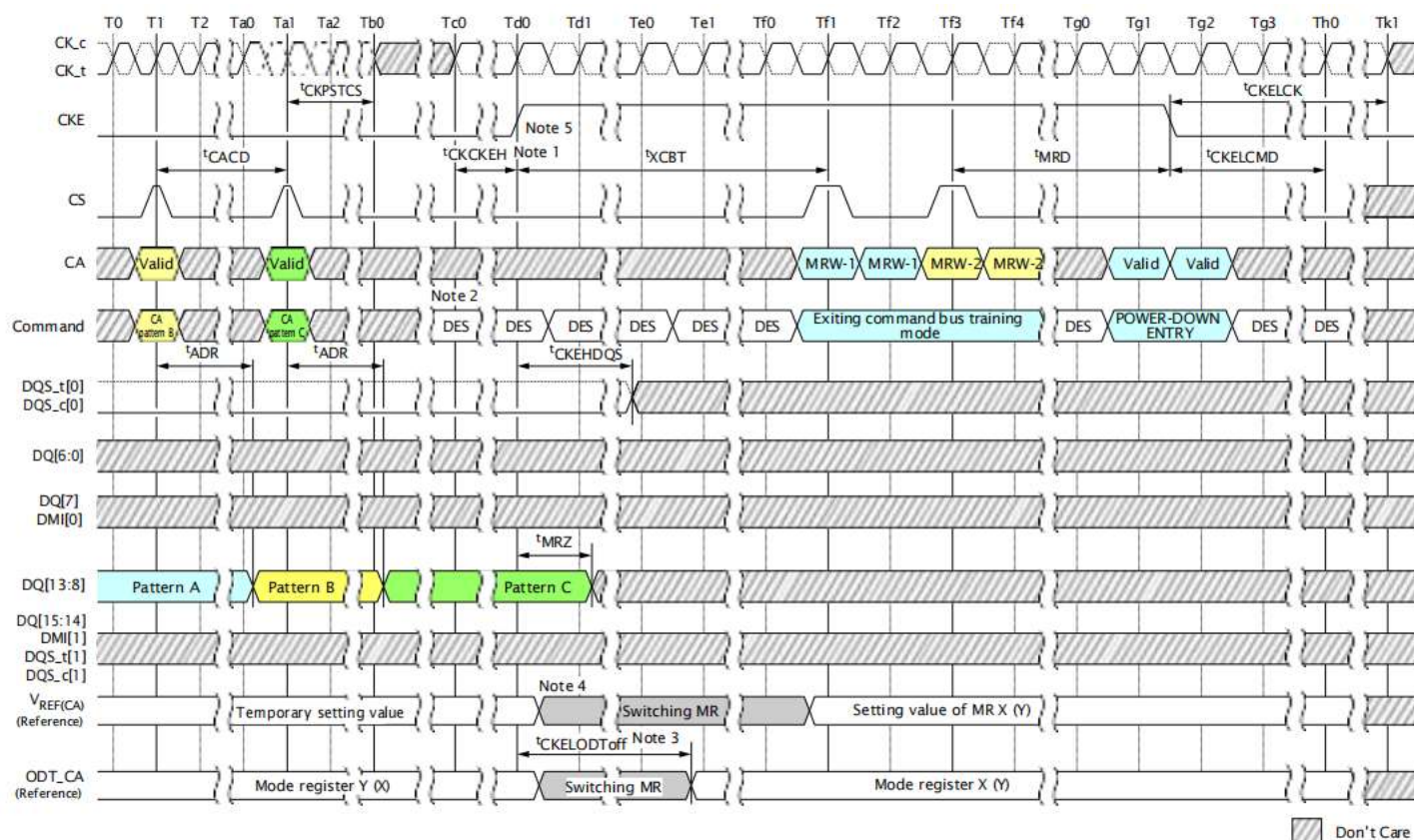
Figure 118: Command Bus Training Mode Exit with Power-Down Entry
