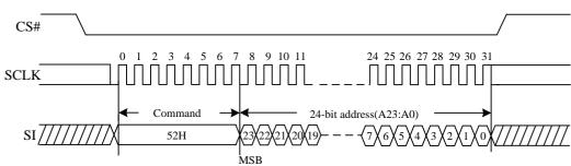
Figure 18. 32KB Block Erase Sequence Diagram
