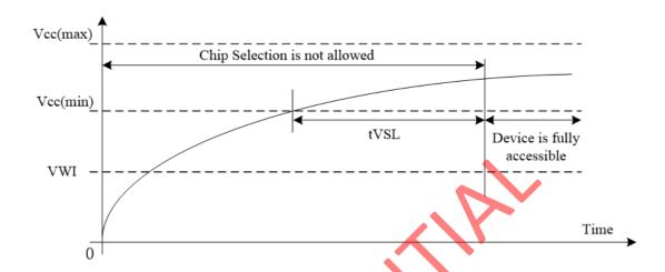
Power-Up Timing and Write Inhibit Threshold
